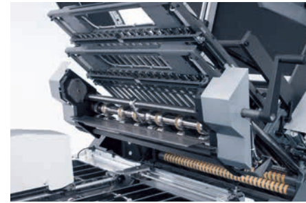
Easy access to the rear-mounted slitter shafts with the lift kit.
