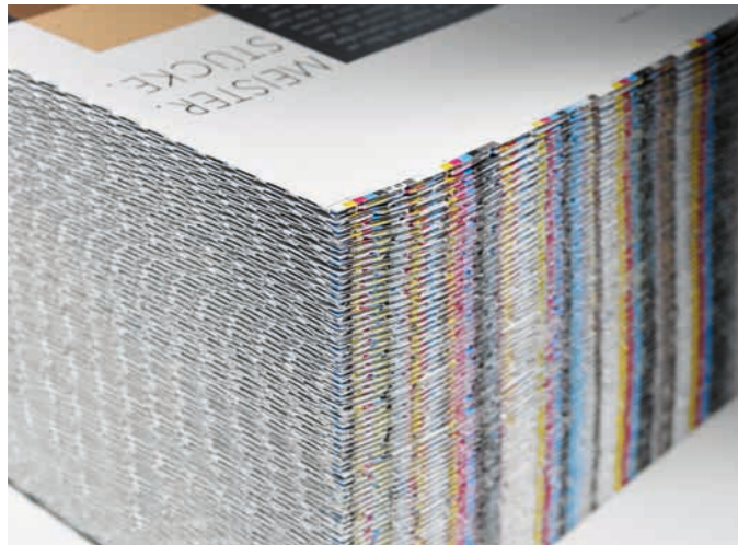
16-page DIN A4 – signature production at the highest level with the Stahlfolder TH 82-P.
